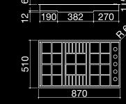
STAINLESS STEEL with cast iron pan supports and burner caps code LABH900
